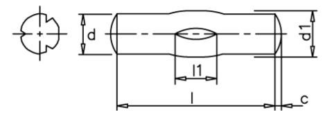
$\begin{array}{ll} d1 &= 4.0 \\ d2 &= 4.15 \\ \text{Length} = 16\text{-}20 \end{array}$
